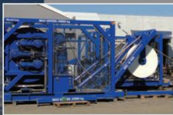
Container integrated handling system
