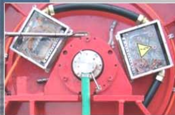
Slip ring installed on winch
